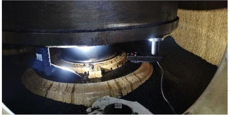
The stroke length and position of the piston is found by using laser.
